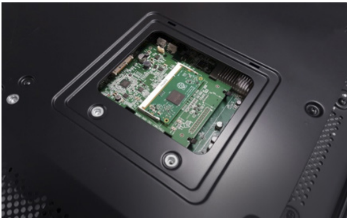
NEC large format display with Interface Board and Compute Module installed
